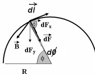
$$d\vec{F} = I(d\vec{l} \times \vec{B}) = I \begin{vmatrix} \vec{i} & \vec{j} & \vec{k} \\ dx & dy & 0 \\ 0 & 0 & B \end{vmatrix} = I B dy \vec{i} - I B dx \vec{j} = (dF_x, dF_y, 0)$$
