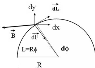
$$\vec{F}_2 = \int_c d\vec{F} = \int_c I (d\vec{L} \times \vec{B}) = \int_c (B dy \vec{i} - B dx \vec{j}) = I B \int_c dy \vec{i} - I B \int_c dx \vec{j}$$
